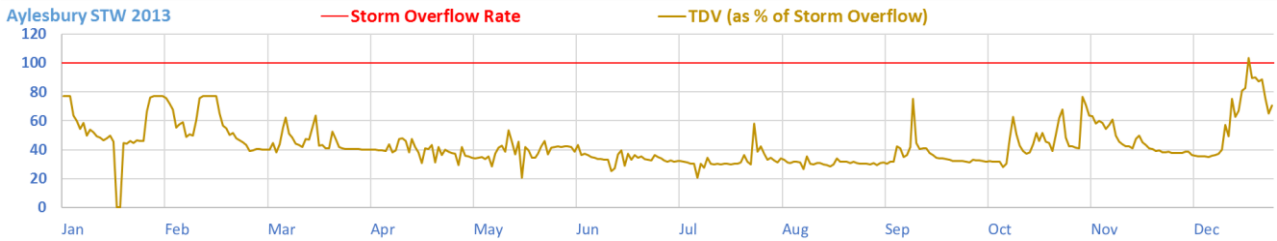
Figure 2: total daily flow curve for 2013 smoothing out the rectilinear, clipped edges of 15-min flow curve in Fig 1
